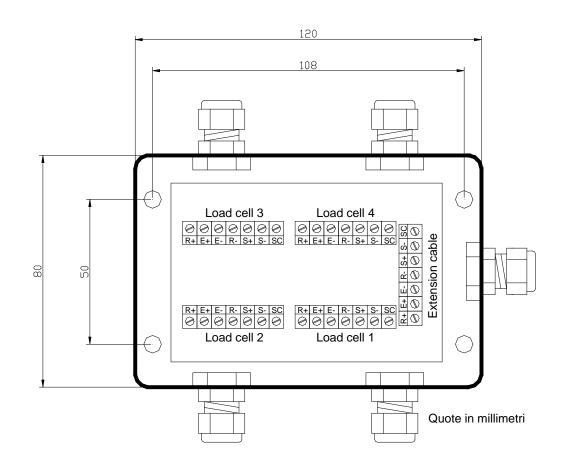
Material: polycarbonate Dimensions: see the figure. Height: 55mm
